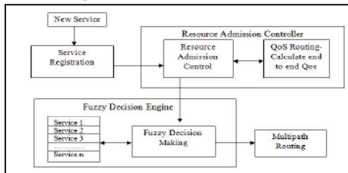
Fig. 3.1 System Design-Block Diagram
