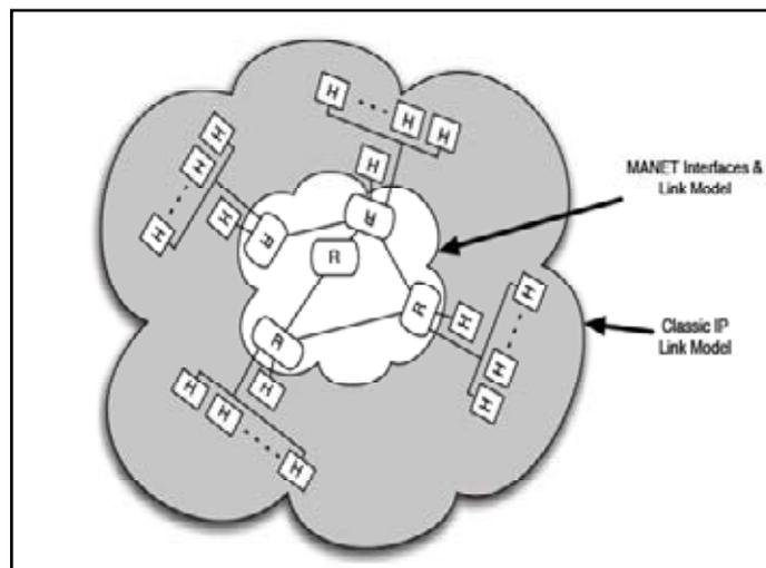
Fig. 1: Configured MANET with routers and hosts
