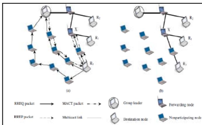
Fig 3.2.1 Node R3Joining in Multicast tree
