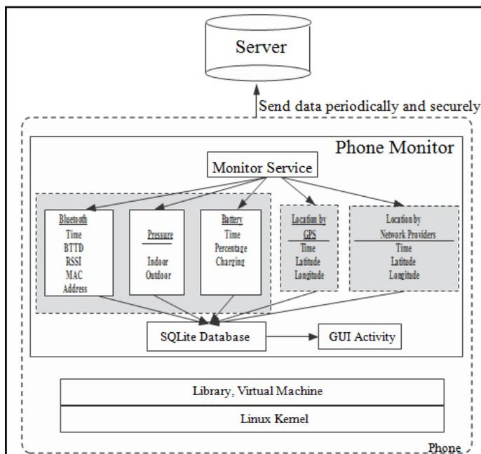
Fig. 2: Software Architecture
