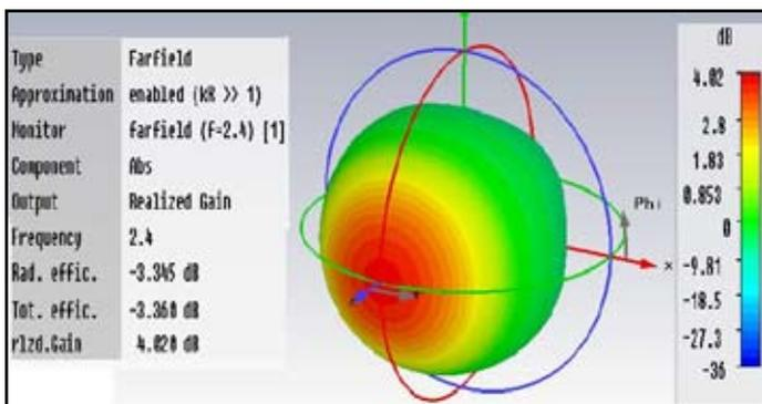
Fig. 8: Gain of Microstrip Dual Patch Antenna
