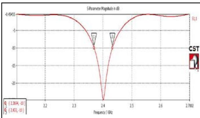
Fig. 7: Return Loss of Microstrip Dual Patch Antenna
