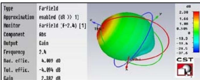
Fig. 3: Simulated Gain Pattern
