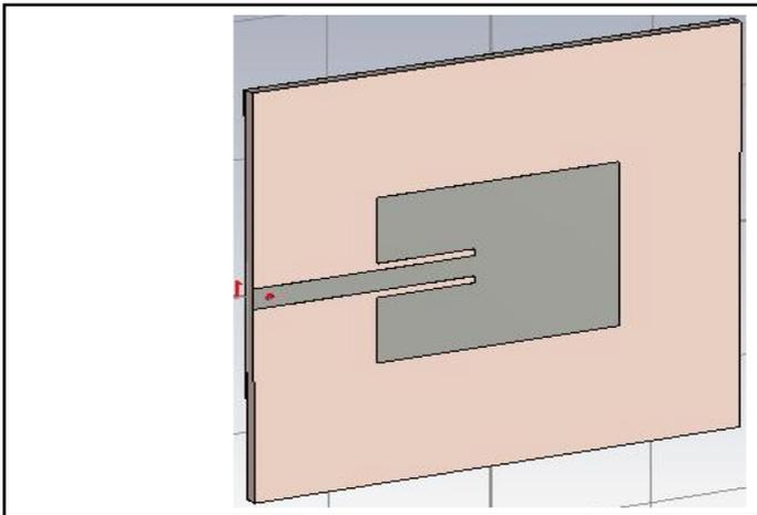
Fig. 1: Microstrip Patch Antenna
