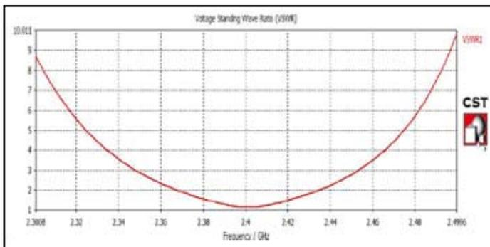
Fig. 9: VSWR Pattern of Dual Patch Antenna
