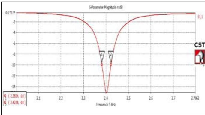
Fig. 2: Simulated Graph of Return Loss
