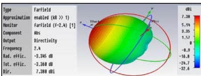
Fig. 10: Directivity Pattern of Dual Patch Antenna
