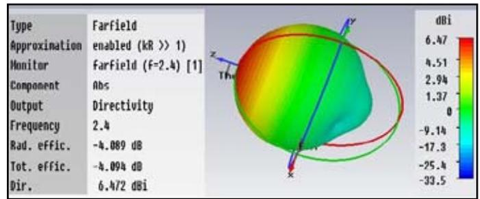
Fig. 5: Simulated Directivity Pattern
