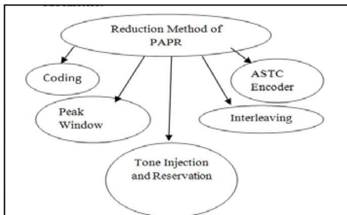
Fig. 1: Method of Reduction PAPR
