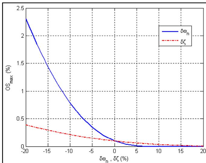
Fig. 2: Effect of process parameters change on system maximum overshoot (Feedback PD compensator for a second order process).
