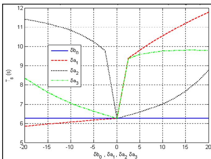
Fig. 4: Effect of process parameters change on system settling time (Feedback PD compensator for a third order process).
