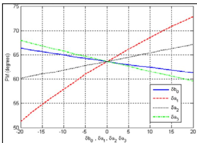
Fig. 6 : Effect of process parameters change on system phase margin (Feedback PD compensator for a third order process).
