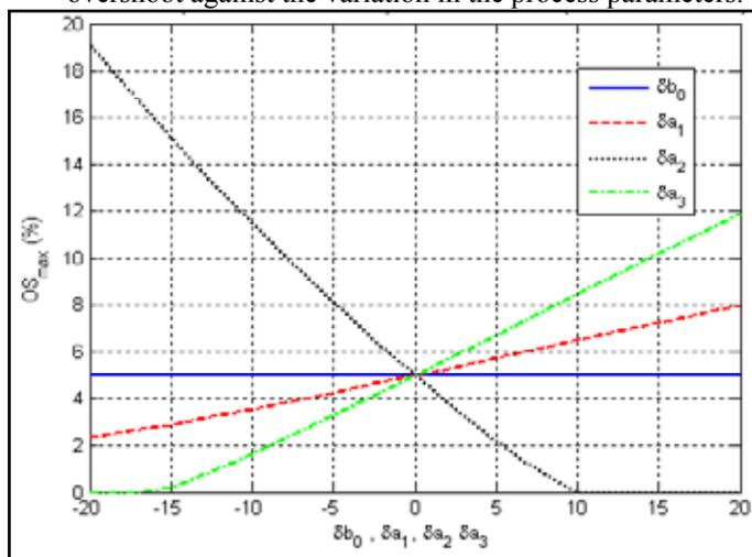
Fig. 5: Effect of process parameters change on system maximum overshoot (Feedback PD compensator for a third order process).
