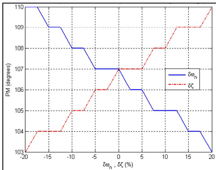
Fig.3: Effect of process parameters change on system phase margin (Feedback PD compensator for a second order process).
