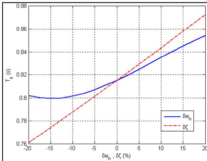
Fig. 1: Effect of process parameters change on system settling time (Feedback PD compensator for a second order process).
