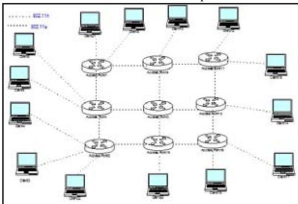
Fig.2: Experimental Setup with Mesh clients and Mesh Access Points
