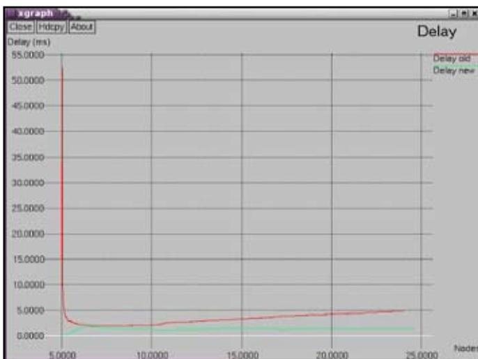
Fig. 4: End-to-end delay of WMN
