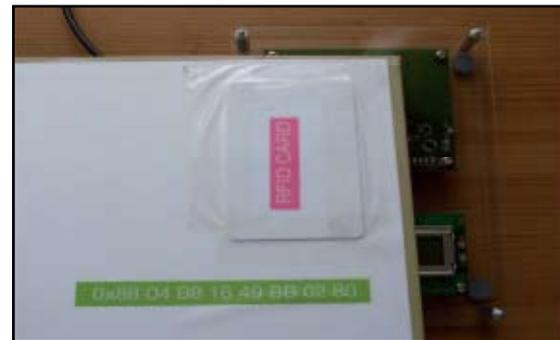
Fig. 4 : Workbook inside cover showing the RFID card (tag) used in the prototype
