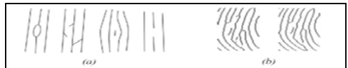
Fig. 4.11 : Thinning step: (a) typical imperfections appeared during the thinning step, and (b) a thinned fingerprint structure before and after removing imperfections
