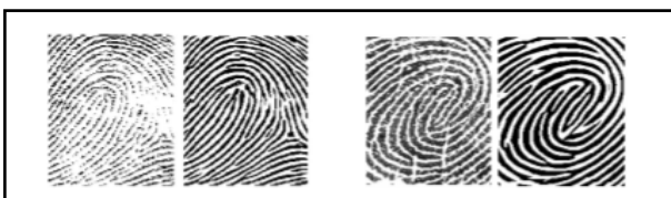
Fig. 4.8 Examples of original and enhanced fingerprint images techniques are commonly used [65, 44, 55, 9, 79, 67].
