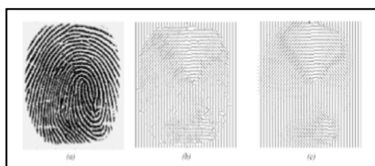
Fig. 4.5 Local ridge orientation of a fingerprint image computed over a square-meshed grid: (a) original image, (b) orientation image, and (c) smoothed orientation image. Each element of (b) and (c) denotes the local orientation of the ridges
